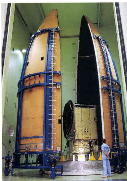
Figure 5. DASA-Dornier (D) and Oerlikon-Contraves (CH) successfully developed the Ariane-5 fairing with its passive noise-control system, shown here with the Olympus test structure used to assess acoustic performance in the LEAF
