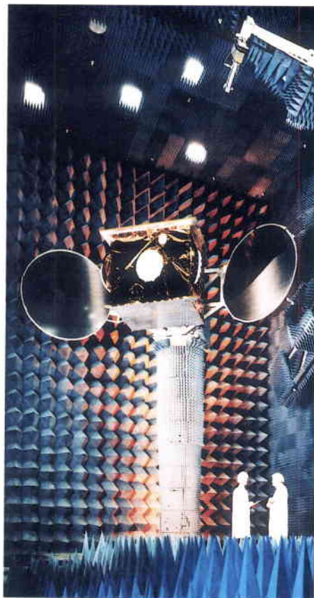
Inmarsat-3 satellite model undergoing antenna tests (photo courtesy of Matra Marconi Space)
