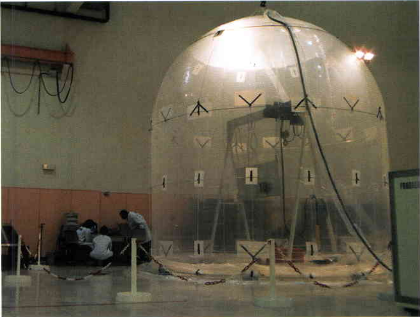
Figure 7. Helium tent used by Matra-Marconi-Space, Toulouse (F) for microvibration studies
