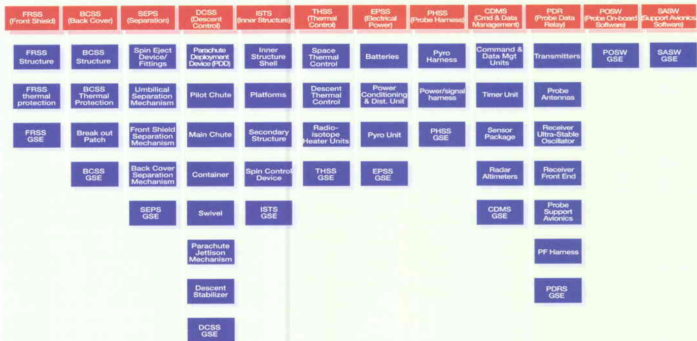
Figure 9. Huygens Probe subsystem breakdown
