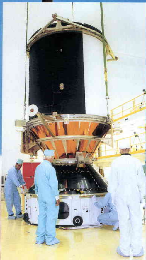
Mating of the upper payload composite, consisting of Maqsat-H and Teamsat, with its flight adaptor in the Final Assembly Building in Kourou, French Guiana
