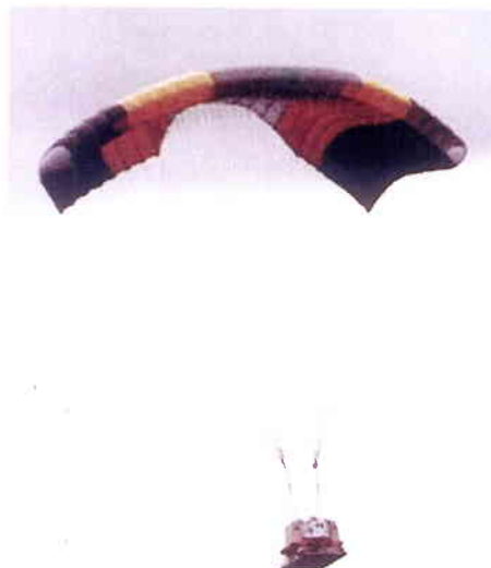
A test vehicle makes the first automatically-guided, parafoil-based descent and landing as part of ESA's Parafoil Technology Demonstration programme through which soft and accurate landing techniques for the planned Crew Transfer Vehicle (CTV) are being validated. ESA is studying a CTV for the transport of international crew to and from the International Space Station (photo courtesy of ESA-Daimler-Benz Aerospace)
