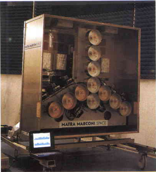
Figure 7. An 11-element L-band MIRAS aircraft breadboard suitable for a Hercules C-130
