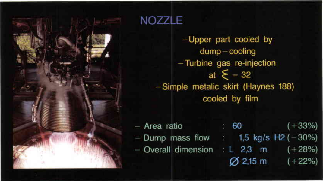
Figure 6. The modified nozzle
