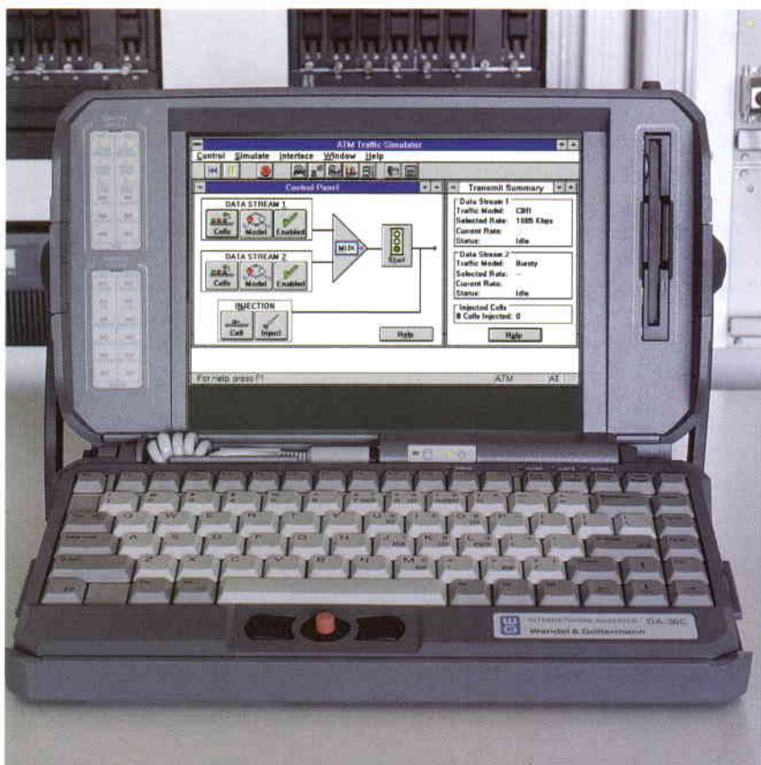
Figure 4. The ATM internetwork analyser
