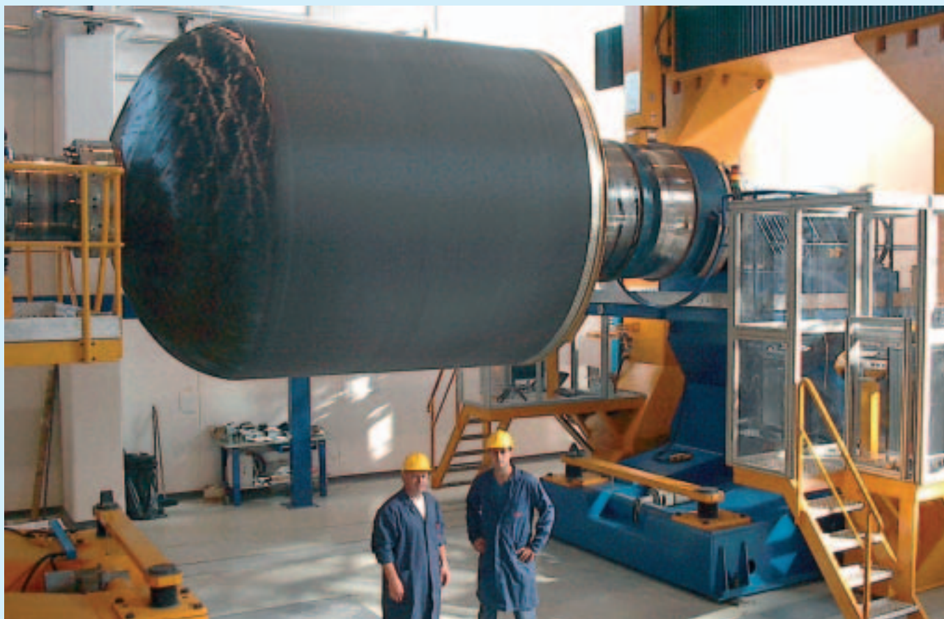
The Technological Model of the Vega first stage's P80 motor during manufacture at the Colleferro factory (photo courtesy of Avio)
