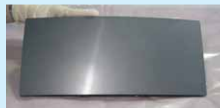
The optical face of the first FM secondary mirror blank for Gaia. The optical surface accuracy of better than 50 µm rms will be improved by polishing to better than 10 nm rms
