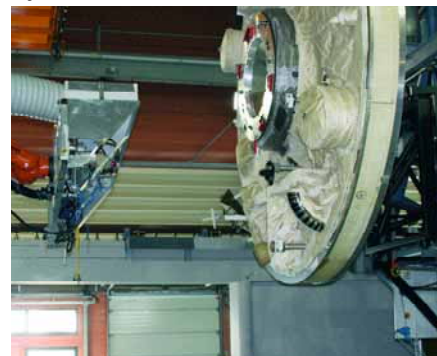
In 2006, ATV's computer and sensors mounted on a mobile platform (left) proved they could approach and dock with the ISS (right) from 250 m out
