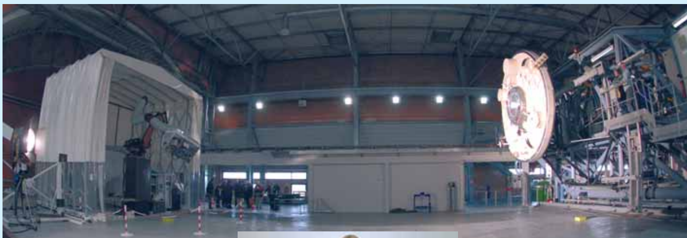
Rendezvous and docking tests were completed in the Val de Reuil facility using a model of the aft of ISS and the ATV sensors
