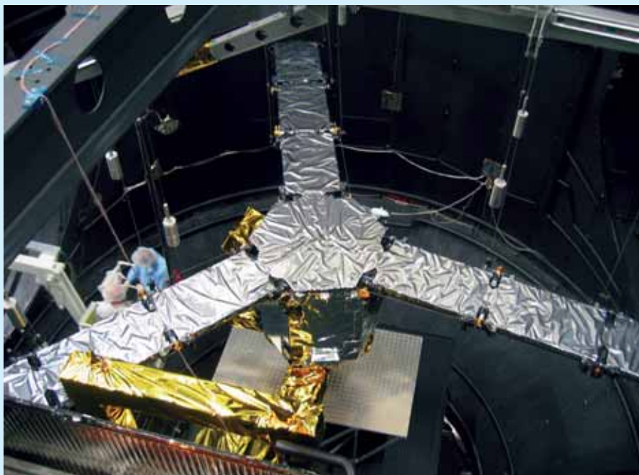
The SMOS payload ready for thermal testing in ESTEC's Large Space Simulator
