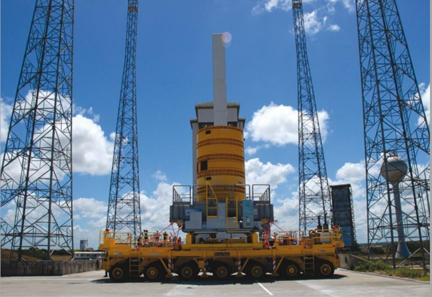
The 'Fardier' specialised transport vehicle in front of the Vega mobile gantry at the Guiana Space Centre, Kourou. The Fardier (French for 'dray' – a vehicle for carrying heavy loads) carries the Vega P80 first stage from the Regulus propellant-loading plant to the launch table. This Fardier is carrying dummy loads, each weighing 20 tonnes, to simulate the P80 during testing of the mechanical systems on the launch table
