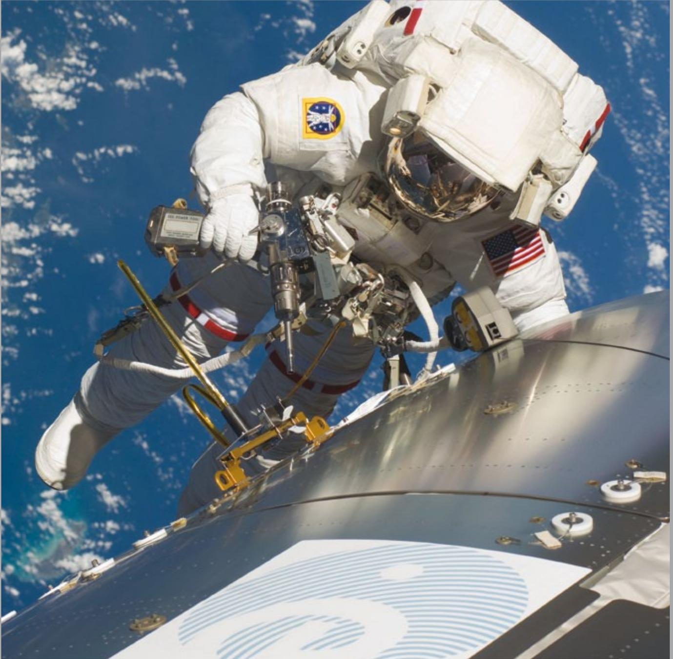
During a six-hour spacewalk on 21 November, NASA astronauts Randy Bresnik and Mike Foreman (out of frame) install the Grappling Adaptor To On-Orbit Railing Assembly, or GATOR, on the Columbus laboratory
