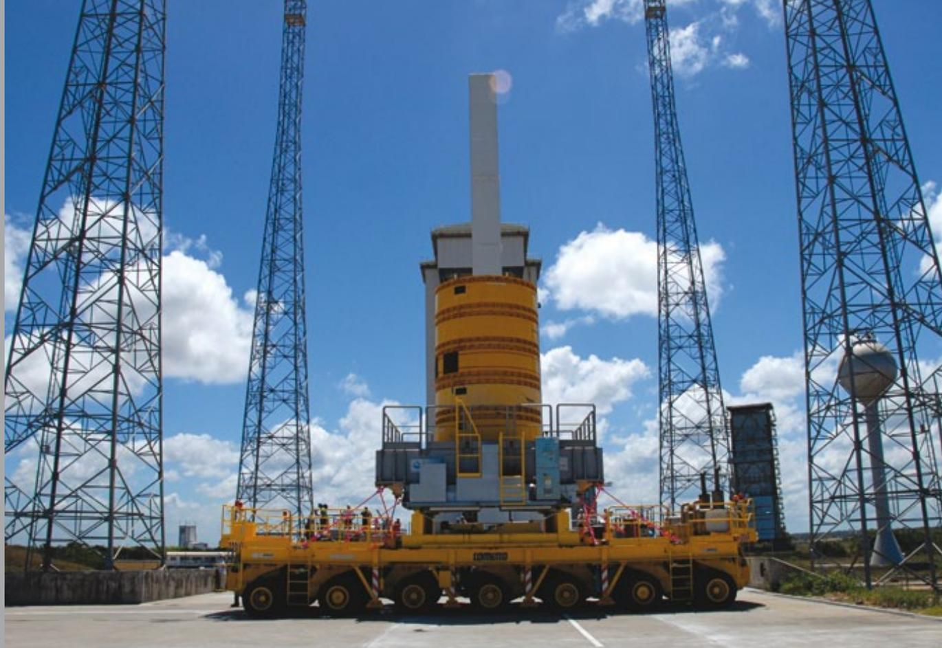
The 'Fardier' specialised transport vehicle in front of the Vega mobile gantry at the Guiana Space Centre, Kourou. The Fardier (French for 'dray' – a vehicle for carrying heavy loads) carries the Vega P80 first stage from the Regulus propellant-loading plant to the launch table. This Fardier is carrying dummy loads, each weighing 20 tonnes, to simulate the P80 during testing of the mechanical systems on the launch table
