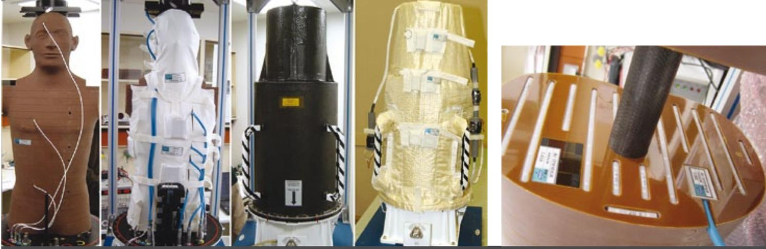
↑ Assembling the Matroshka phantom, left to right: anthropomorphic upper torso equipped with active and passive detector systems; torso with poncho and hood equipped with passive detector systems for skin dose measurements; carbon-fibre container to simulate the astronaut's spacesuit; facility ready for launch, equipped with multi-layer insulation for thermal protection
