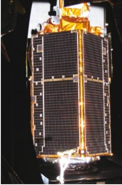
The reason why the SIRAL was non-redundant was simply down to cost. The radar represented a significant portion of the overall cost and providing an onboard spare would have exceeded the strict limit on cost placed on the mission. This decision was hotly debated during the development phase, and it was perhaps this debate that triggered one comment after the launch failure, that “Non-redundancy saved us quite a lot of money!”
