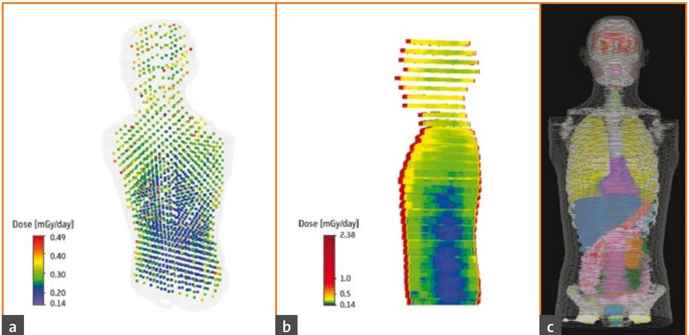
↑ a: depth dose distribution of absorbed doses measured with TLDs inside the human phantom; b: inclusion of the absorbed doses measured with the poncho detectors; c: location of organs based on the Zubal phantom
