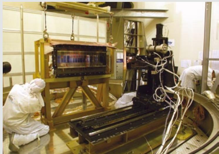
The Gaia Focal Plane Assembly engineering model being prepared for the functional tests at Astrium SAS (Toulouse)
