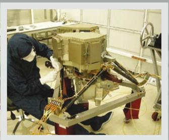
MIRI instrument ready for vibration test
