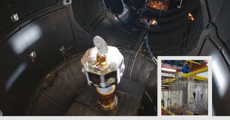
BepiColombo MMO Thermal Model in the Large Space Simulator at ESTEC
