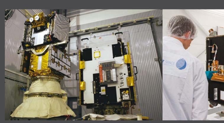
↑ Bigger than SMOS? From this perspective view, Proba-2 in the foreground seems bigger than its much larger cousin, the SMOS satellite, seen mounted on its launcher adapter (Proba-2 fits inside this structure)
