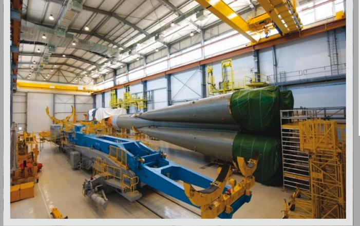
In French Guiana, the first Soyuz for launch from Europe's Spaceport has been assembled in the MIK building. The vehicle will then be transferred to the launch pad in the horizontal position on a rail-mounted erector system, seen left. At the pad, the erector will raise the Soyuz into the upright position for launch
