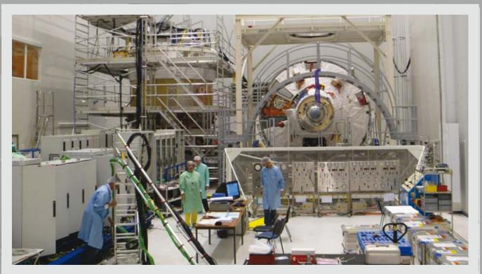
The mating of ATV *Johannes Kepler*'s Service Module and the Integrated Cargo Carrier took place at the end of October. Here, all the components are being prepared for mating in the S5C hall at Kourou, French Guiana
