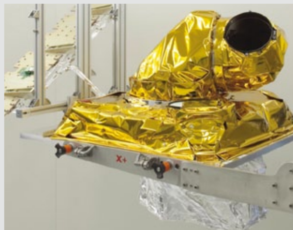
Alphasat Technology Demonstration Payload 1, the Laser Communication Terminal
