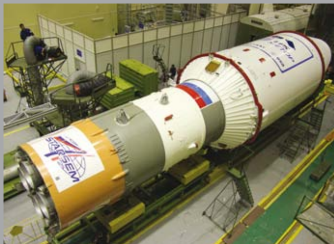
Five days before launch, MetOp-B is inside the fairing connected to the third stage of the Soyuz rocket, ready to be integrated with the first and second stages
