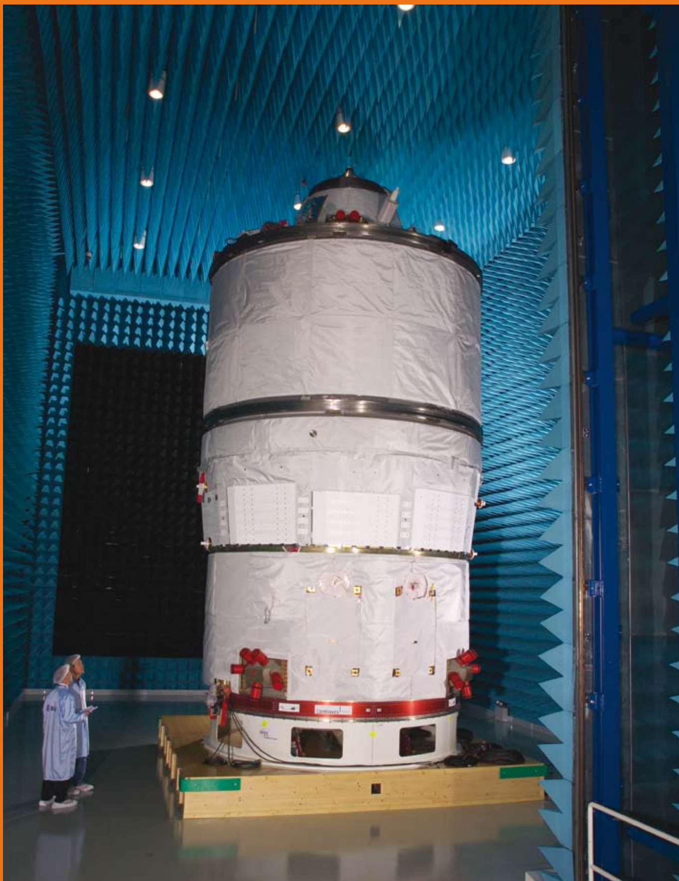
↑ ATV Jules Verne inside ESTEC's Maxwell chamber for electromagnetic compatibility and interference testing in 2004
