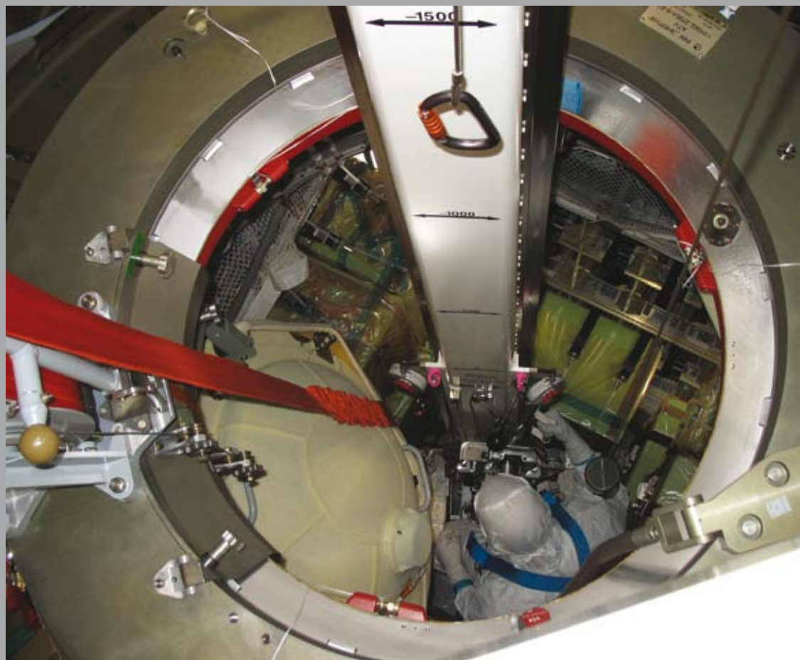
Test inside ATV Albert Einstein (ATV-4) of the new Late Cargo Access Means (LCAM) in Kourou. The new LCAM will allow larger and heavier last-minute cargo to be loaded, 75 kg of Triple Cargo Transfer Bags instead of the previous capability of 25 kg Double Bags
