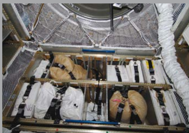
One of the last images taken inside ATV Edoardo Amaldi by the ISS crew just before hatch closure and undocking. The location of stowed waste was documented before departure to verify centre-of-gravity calculations (NASA/ESA)
