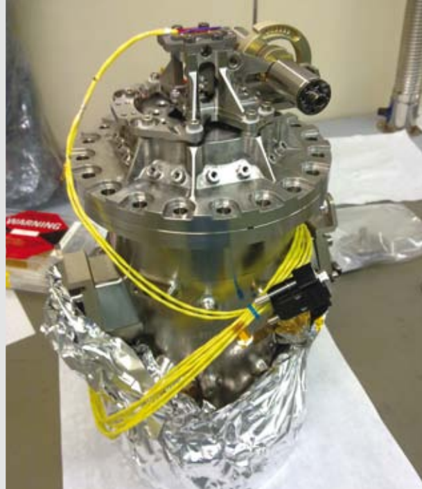
LISA Pathfinder: a Development Model of the actuator for the launch lock eight fingers sits on top of the Qualification Model of the Vacuum Enclosure after a fit check. Inside already sit the various mechanisms and the test mass
