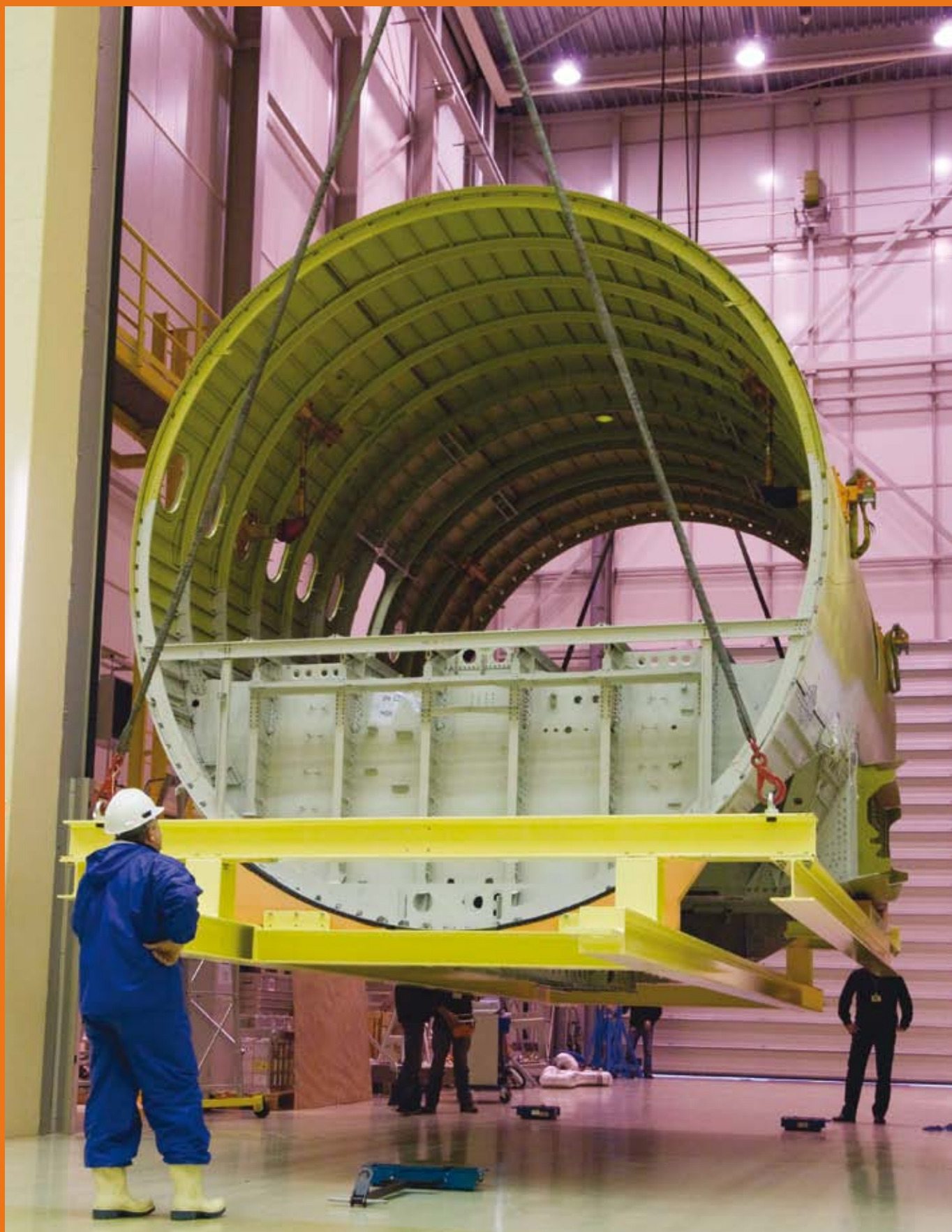
↑ Demonstrating how ESTEC is also able to serve wider European industry, Airbus completed a complex set of vibration tests on a fuselage section using ESTEC's largest vibration facility, called Hydra, in 2010
