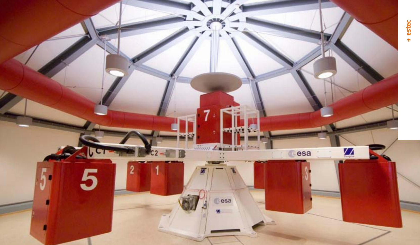
↑ The Large Diameter Centrifuge, run by the Life and Physical Sciences Instrumentation and Life Support Laboratory of ESTEC, now made available for scientists interested in artificial gravity effects
