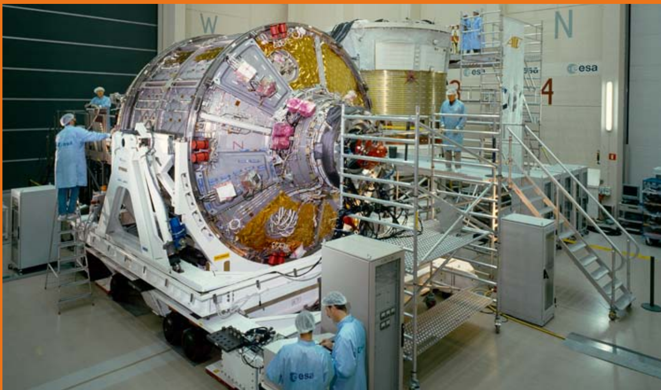
↑ ATV Jules Verne undergoing preparation for testing in the clean one word room outside the Large European Acoustic Facility (LEAF), the largest test facility of its kind in Europe
