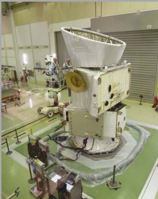
BepiColombo in integrated launch configuration on the vibration table at ESTEC
