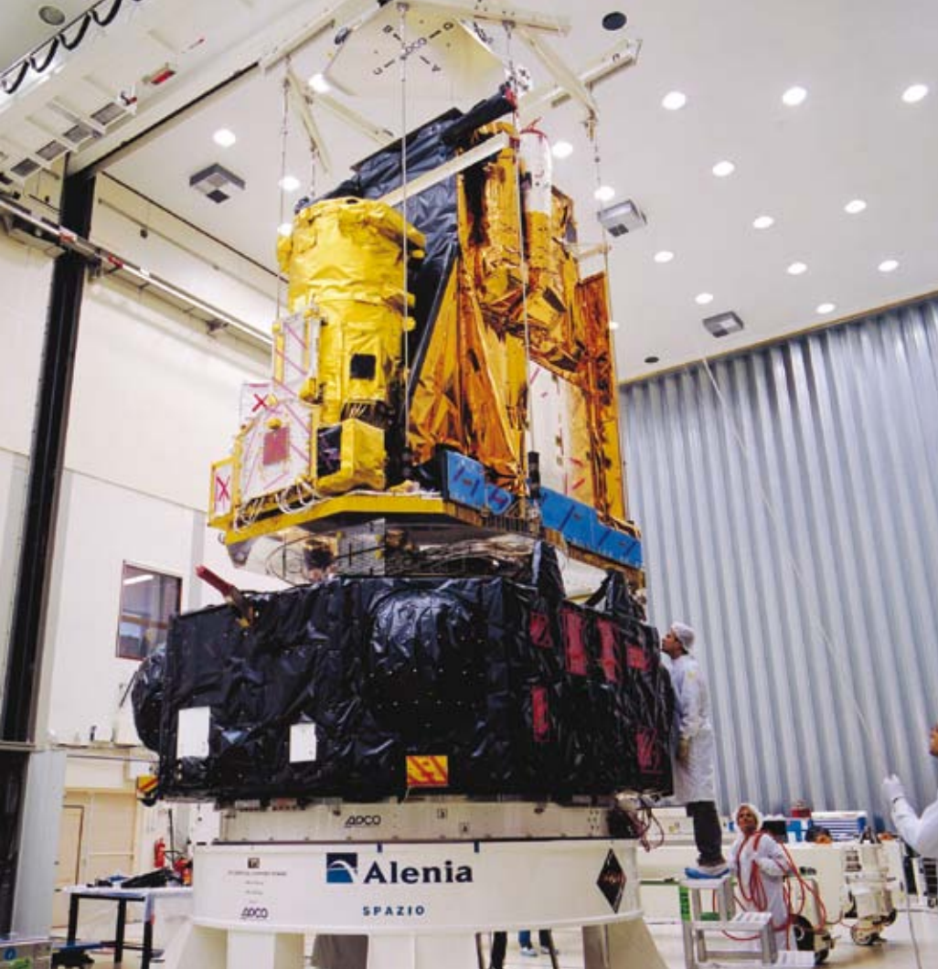
↑ ↗ The Integral Structural/Thermal Model during testing at ESTEC in 1998, (centre) in the Large Space Simulator and (right) in the Large European Acoustic Facility test chamber
