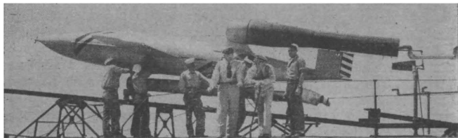
With four jato takeoff units, the Loon, improved version of V-1, needs a launching ramp only slightly longer than itself
