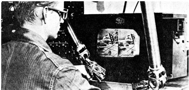
Same type of "manipulators," but observation is by means of television. The double image on the screen becomes a three-dimensional picture when viewed through polarized spectacles (Oak Ridge National Laboratory)
