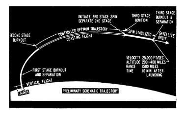
The official schematic drawing of the satellite shots. The term "range 1500 miles" on the diagram refers to the expected impact point of the second stage, about 1500 miles from the takeoff site.
