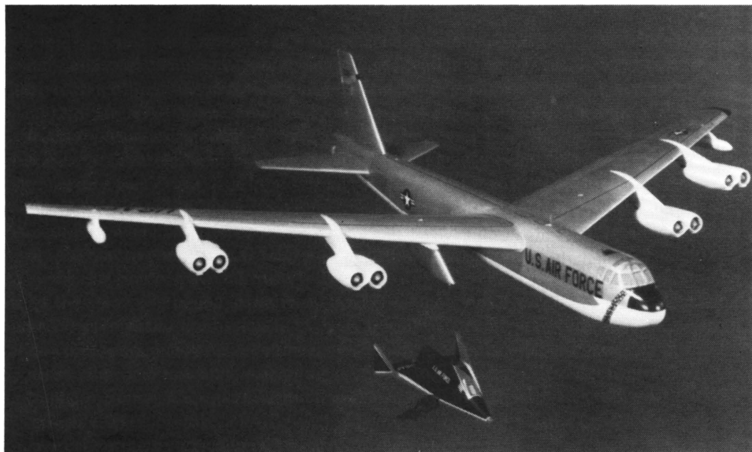
Figure 4 Scale models showing an early Dyna-Soar design being air-dropped from a B-52 (photo courtesy: Boeing Aerospace).
