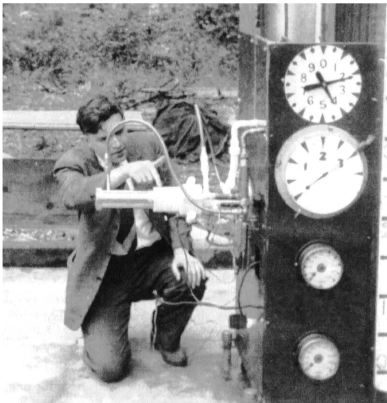
Figure 5–11: Wyld, after a static test of RMI motor M16-G on 20 September 1942, probably taken at their plant at Pompton Plains, New Jersey. Note the frost on the cooling jacket and “borrowed” elements from ARS Test Stand No. 2, including the clock and other dials. The M-16 designation mostly likely originated from Wyld’s final version of his first successful regeneratively-cooled motor, the M-15, or “Motor 15.” In other words, RMI’s motors were successively improved variations of the original Wyld motor, and included sub-variations, and hence the M16-G model. Smithsonian Photo 78–18197.
