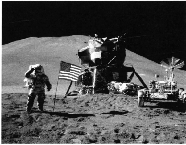
Figure 19–10: A well-known photo of Apollo 15 LM pilot Jim Irwin saluting next to old glory. It is easy to tell that the LM ( Falcon ) is on an incline, which made it difficult to unload the Lunar Roving Vehicle.
