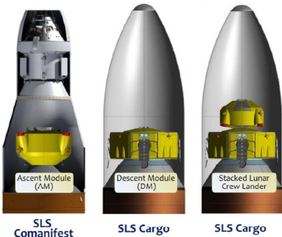
Figure B-1 Elements of Boeing Lunar Architecture Take Full Advantage of SLS TLI Mass and Volume Capabilities
