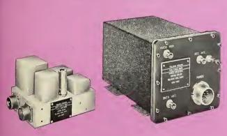
New superheterodyne S-Bond Beocons for guided missile ond drone-control applications. These receivers feature light weight, smoll size, excellent reliability, ruggedized construction.
