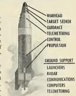
Bendix furnishes mojor elements for missiles af oll types. This illustration represents no particular missile, but shows the general lacation of various airborne Bendix systems and their components. In addition, Bendix produces the Ground Support systems indicated abave.
