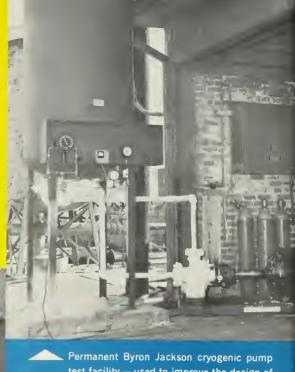
Permanent Byron Jackson cryogenic pump test facility — used to improve the design of pumps and seals and to investigate the effect of suction pressure on pump cool down time.
