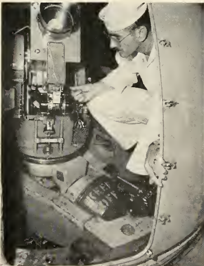
CAMERA ASSEMBLY of the Farrand star tracker is important part of FBM system.
