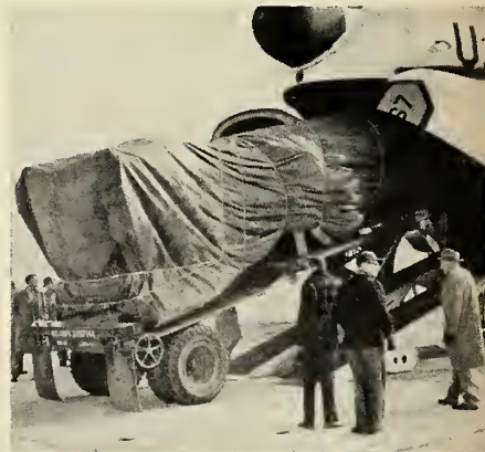
AIR TRANSPORT of missile is another reason for determining center of gravity.
