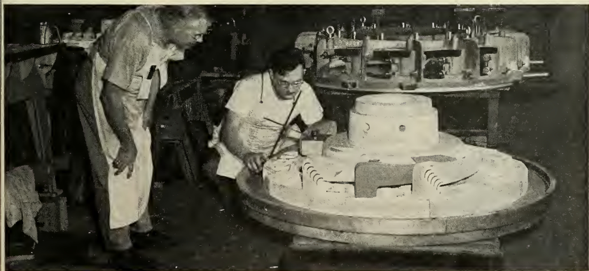
All pattern equipment is carefully checked for accuracy in the foundry pattern shop.
