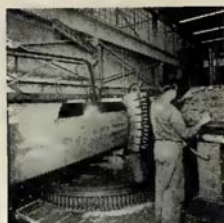
COVER: Alloys for Atlas are formed with Bath Company's "skin-stretching" machine. (p. 24)
