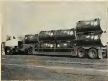
Harco Containers with integral Harco stores trailer can be return-shipped in 1/2 the space required for conventional containers.
