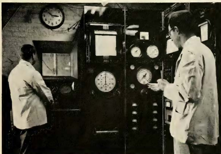
LARGE CONTROL panels automatically start the firing of rocket motors. The panel also records the test results. Pat Howard and Bill Simpson watch the test. The company has built two modern chemical laboratories to expand high pressure work.
