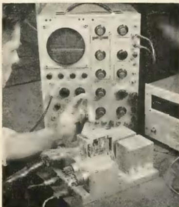
A COMPLETE mixed-input (high and low level) multicoder shown on test bench. The engineer adjusts a modular keyer.
