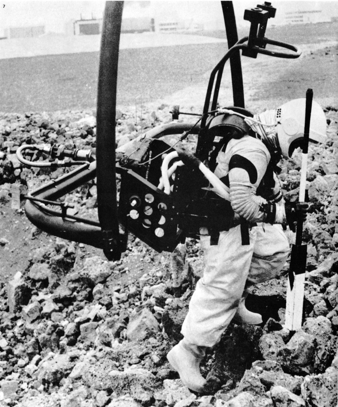
7 Wearing an Apollo pressure suit and buoyed by apparatus that cancels out five-sixths of his weight, an engineer carries out an experiment in a simulated lunar crater.
