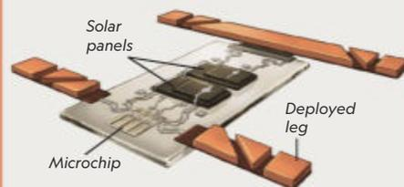
Sections of rigid material restrict bending to predetermined origami-like folds to achieve the desired 3D position. The microchip brain coordinates limb movements to form an autonomous walking robot.
