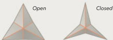
Each shading device is made of fiberglass mesh and weighs about 1.7 tons. Sun-tracking software controls the opening and closing sequence according to the sun's position.
