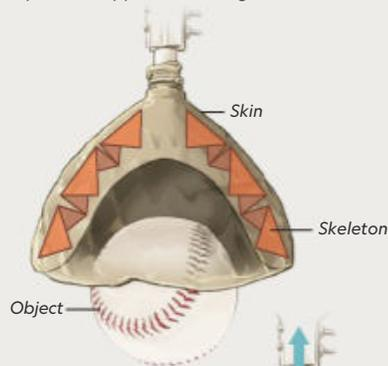
When a vacuum sucks air out of the skin, the origami skeleton collapses along fold lines to grip the enclosed object. It can lift up to 25 pounds—over 120 times its own weight.
