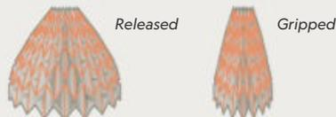
The bell-shaped gripper has a foldable, silicone rubber skeleton based on an origami pattern that can shift between a spherical and a cylindrical shape. It's wrapped in an airtight rubber skin.
