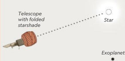
Flying in tandem with a space telescope, the starshade would use thrusters to position itself 31,000 miles in front of it, covering a star that can blaze 10 billion times as bright as its exoplanets.
