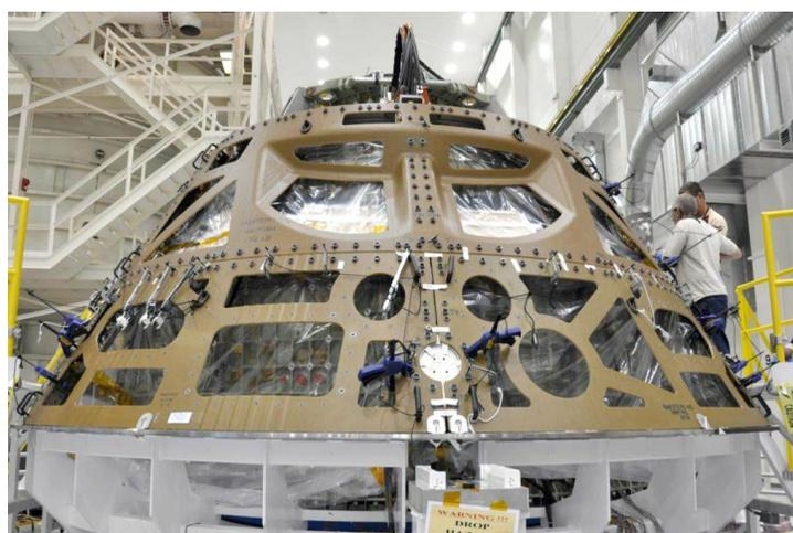
The second series of EFT-1 Crew Module/Service Module retention and release shock tests were completed with the separation bolts performing nominally. This series of tests was used as a qualification test for Environmental Control and Life Support System hardware, as well as the retention and release separation spring assemblies.
