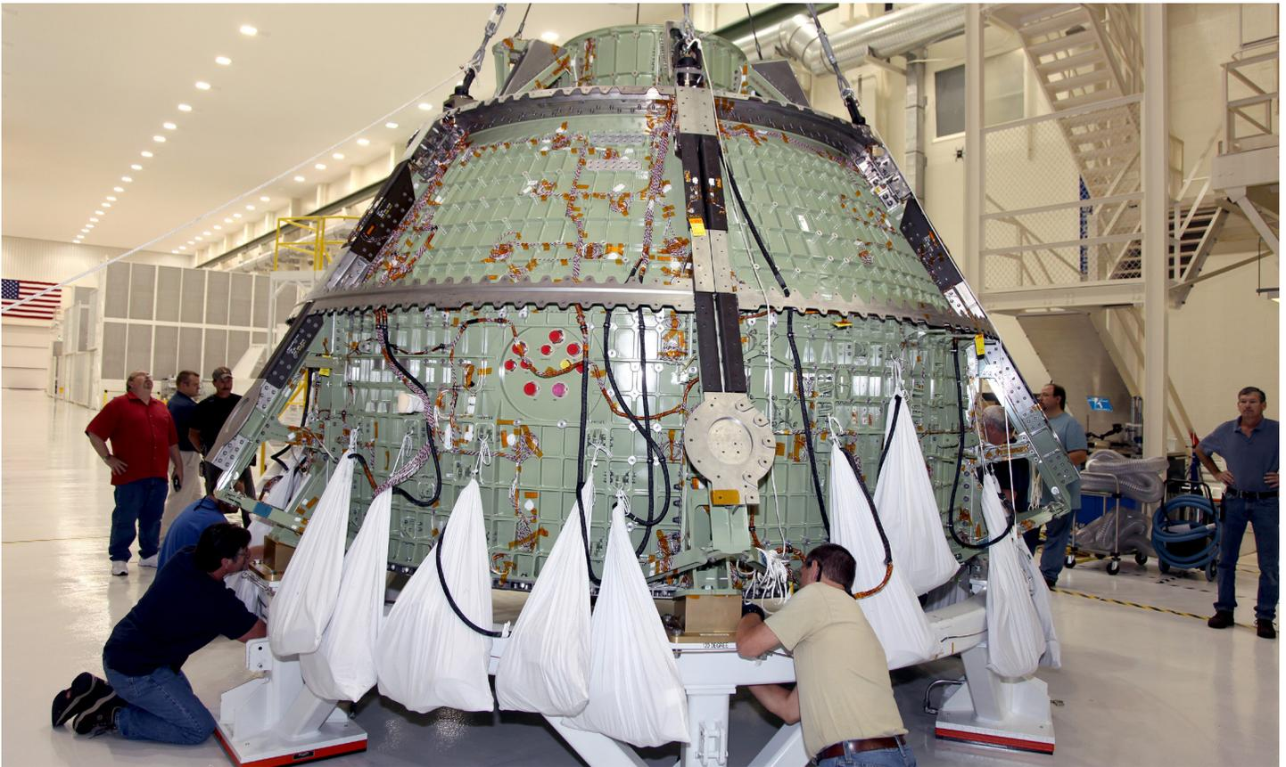
Orion's assembly, integration and production phase officially commenced in June with the arrival of the last of the ECLSS (Environmental Controls & Life Support Systems) elements. In addition, more and more components for all 14 of the spacecraft's subsystems continue to arrive on dock at Kennedy Space Center's Operations and Checkout facility in Florida every day.
