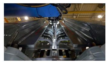
At NASA's Michoud Assembly Facility in New Orleans, engineers used large tooling structures to help them weld together Orion's cone panels using friction-stir welding.
