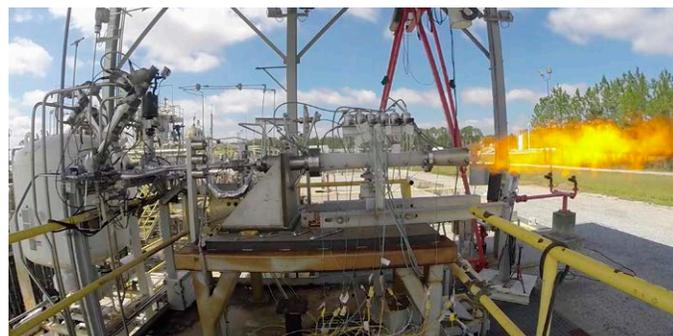
In late 2015, Stennis engineers completed a series of tests on a subscale diffuser system, providing valuable data for the final development testing of the engines that will provide the power Orion needs for deep-space missions.
