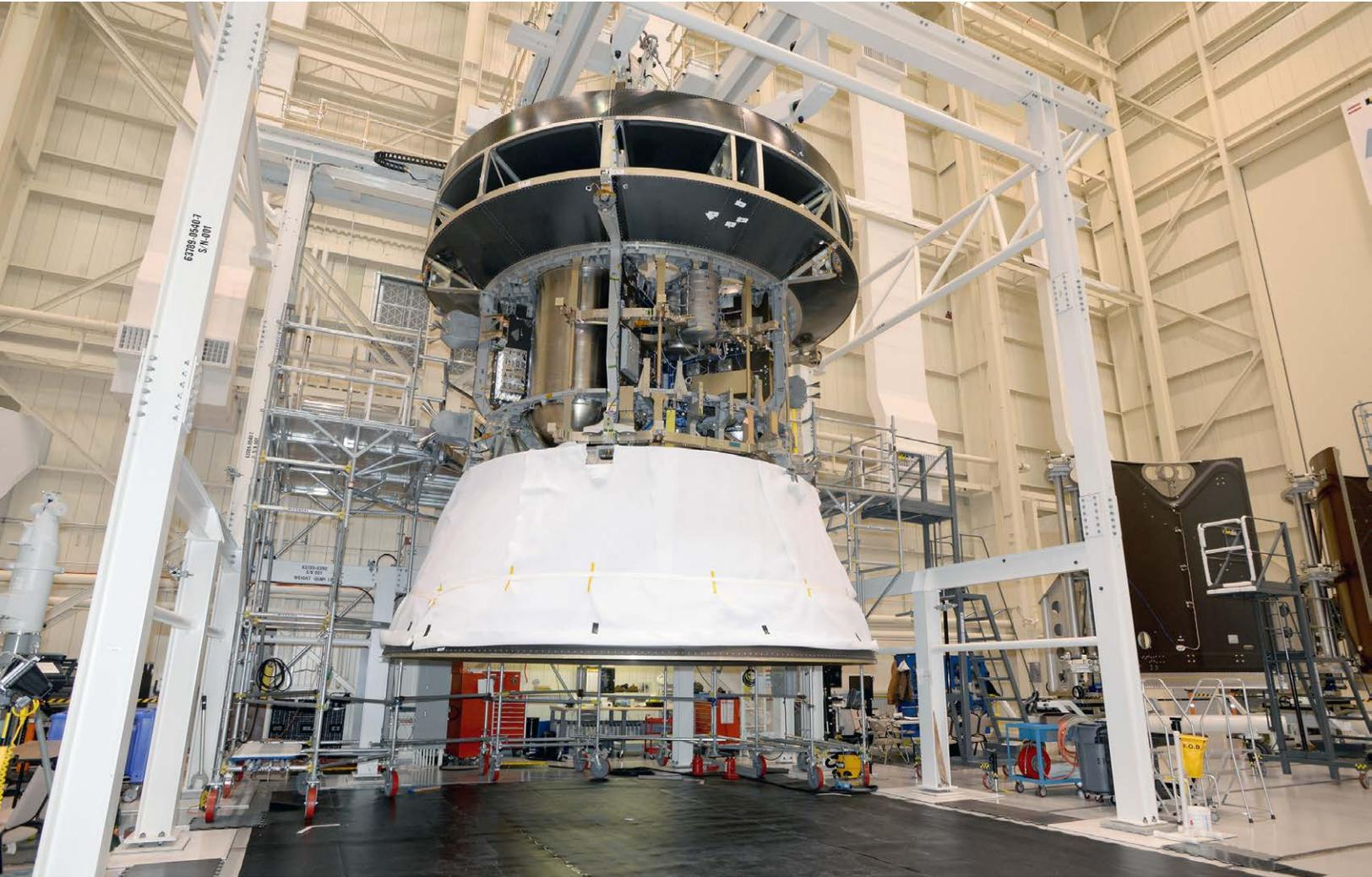
The Orion team at NASA Glenn Research Center's Plum Brook station in Sandusky, Ohio, successfully tested mating operations that will connect the spacecraft's service module to the crew module adapter.
