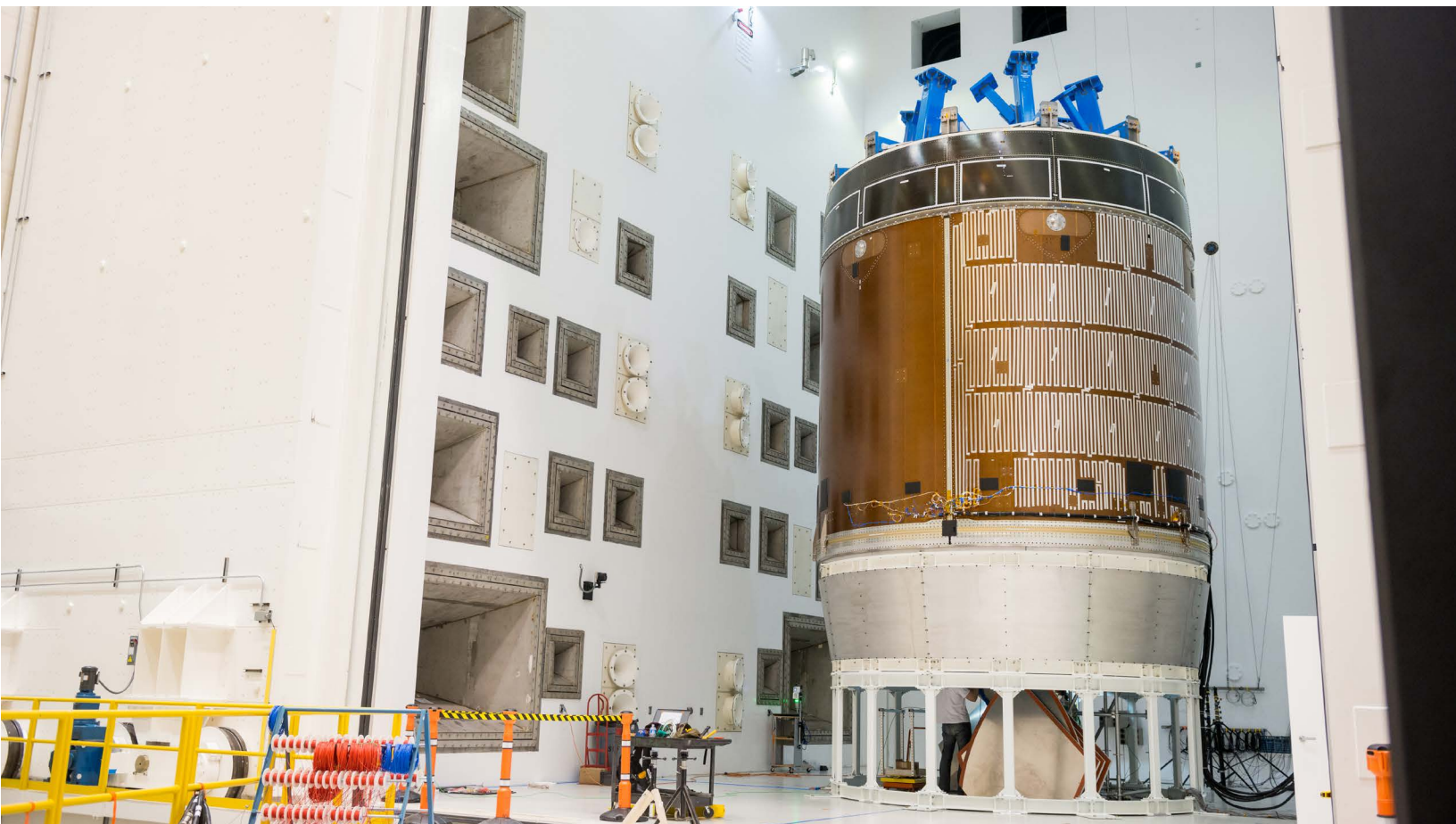
Pictured above: The service module test article sits in the RATF at Glenn's Plum Brook Station ahead of testing. The blue structure sitting on top of the test article is a mass simulator that represents the Orion crew module.
