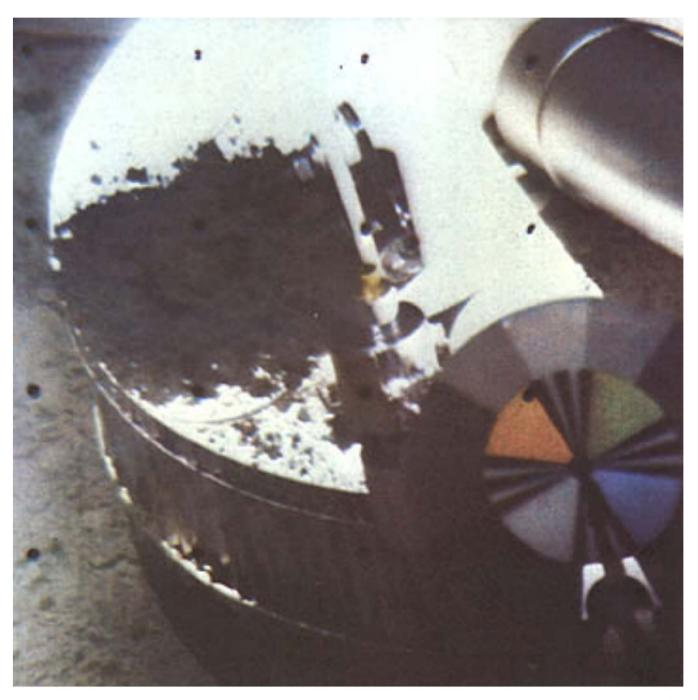
portion of lunar soil, placed on the footpad by the surface-sampling instrument; the attitude-control jet. with its gold-tipped nozzle contrasting with the gray of the lunar soil; and, lastly, a photometric target, consisting of several shades of gray as well as three colors.
