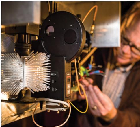
◀ **NIROSETI** The near-infrared/optical instrument mounted on the Nickel 1-meter telescope at Lick Observatory didn't find nanosecond-long pulses expected from far-off lasers, but its field of view was small.
