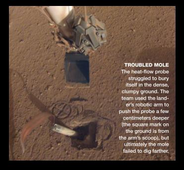
Insight carried three main scientific instruments: A seismometer to record marsquakes, a thermal probe to measure the heat escaping from the planet, and a tracking device to study the orbit of Mars with exquisite precision. It also had a robotic arm to put the instruments on the ground, two cameras, and a wide array of sensors to measure wind speed, atmospheric pressure, local magnetism, and other environmental parameters.
