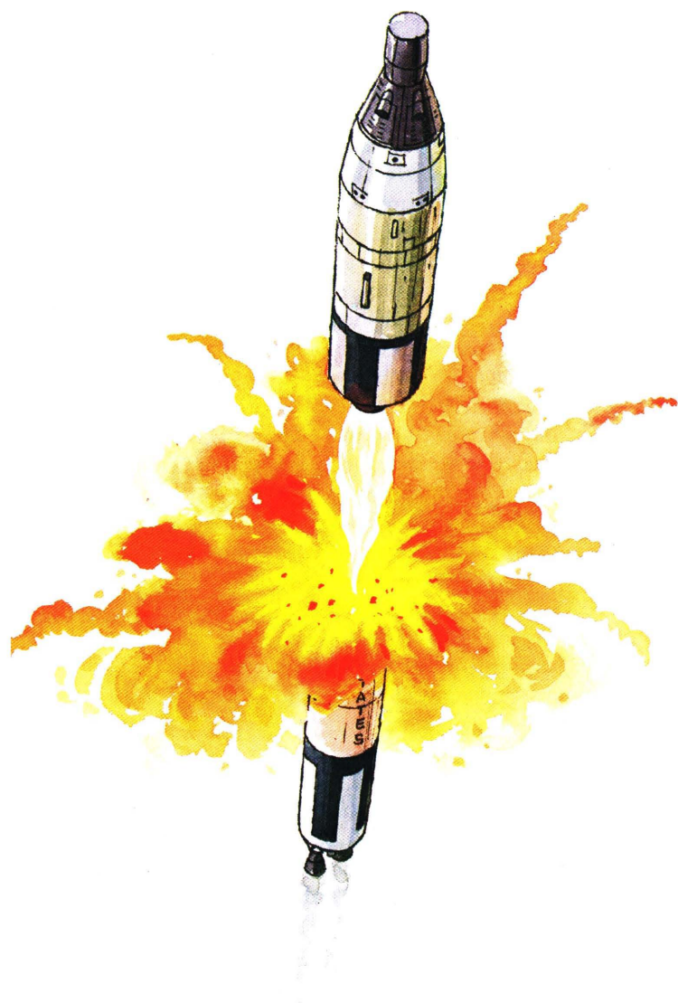
"The second-stage engine has blasted the top of the first stage, causing the oxidizer tank to explode."
