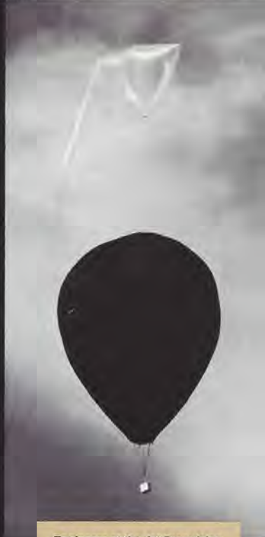
Engineers at the Jet Propulsion Laboratory are already experimenting with double balloon concepts. The clear sack on top is filled with helium; warmed by the Sun, the black balloon below fills with hot air and rises. Photograph: Ed Hauptmann
