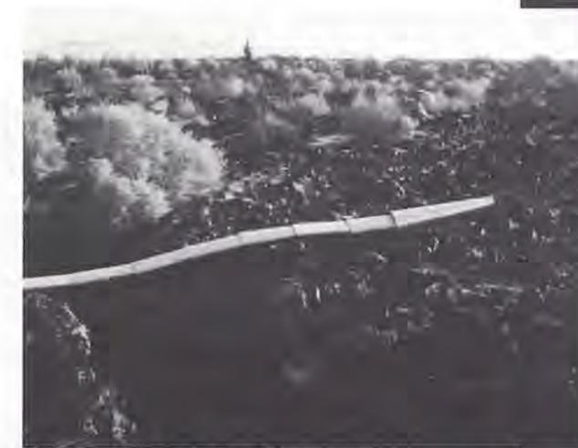
**ABOVE:** The SNAKE successfully traverses a lava crevasse in this 1987 drag-test. The balloon team sought out the harshest and most Mars-like sites to test the SNAKE's ability to avoid snagging on obstacles. *Photograph: Ed Hauptmann*
