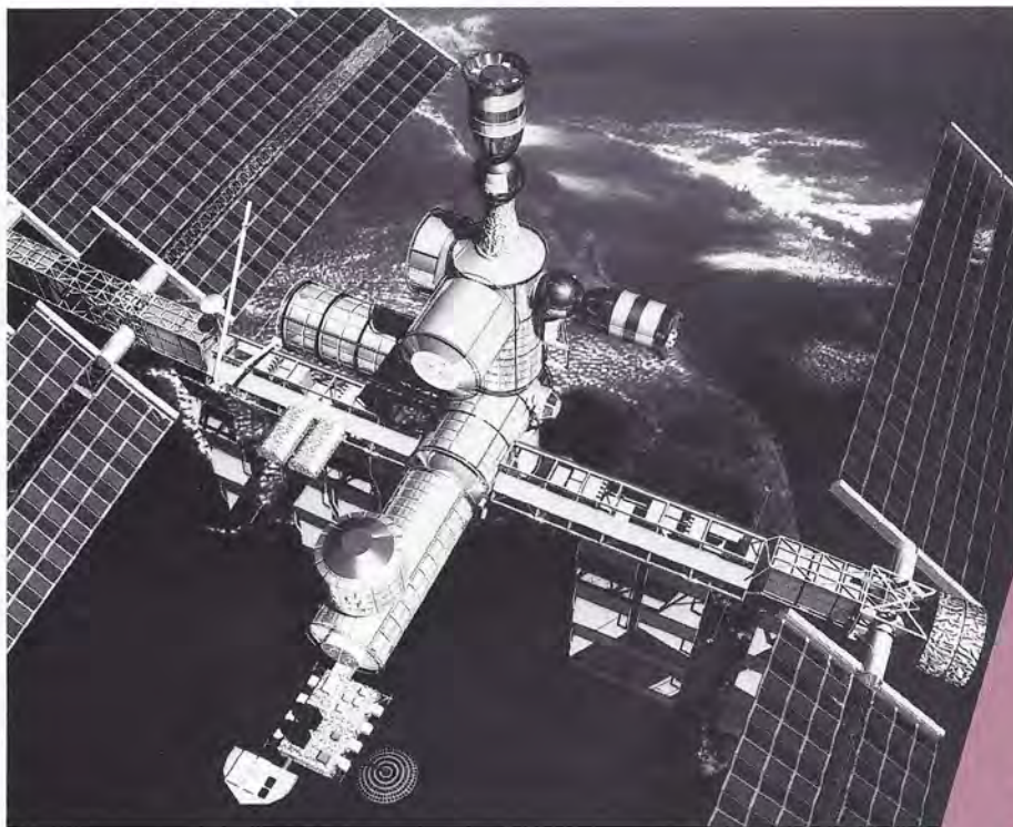
After the recent redesign, the Clinton administration adopted this space station design, called Option A. Note the Russian modules attached to the habitation module at the top of this picture.
