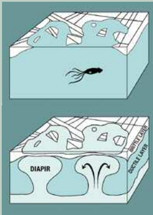
These diagrams show how the thickness of Europa's ice shell is critical to what takes place underneath. In a thin-shell model (top), the liquid ocean beneath can easily melt through the ice or seep up through cracks to the surface. These breaches in the ice shell might allow enough weak sunlight through for photosynthetic sea life to evolve.
