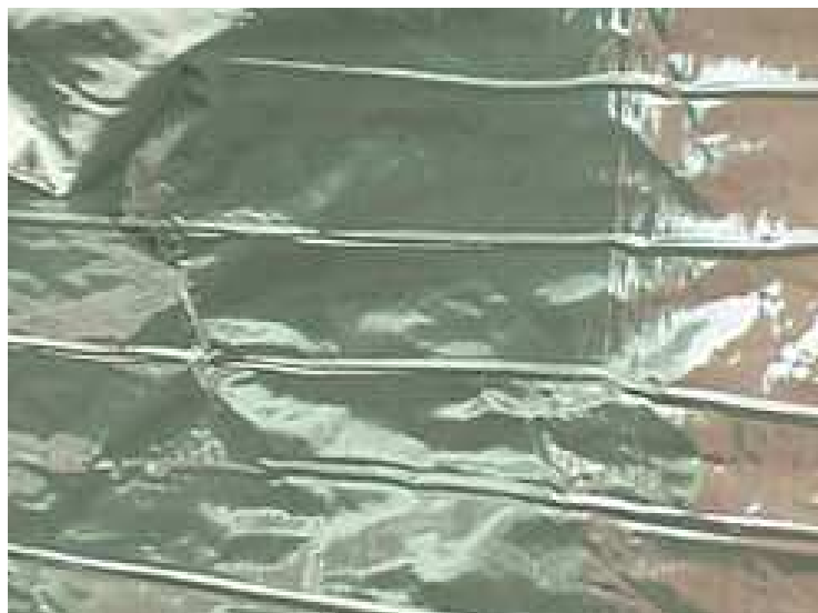
These close-ups show the difference in reflectivity of both sides of the Cosmos 1 solar sail film. The shinier side (top photograph) is coated with aluminum and will reflect 80 to 90 percent of the light that hits it, producing thrust for the spacecraft.
