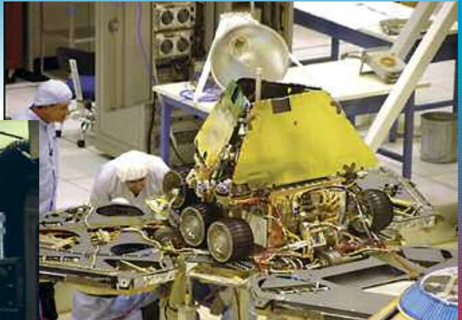
Above: One of the many tests the spacecraft underwent before launch was a check of the landers' deployment mechanisms. Photo: JPL/NASA
