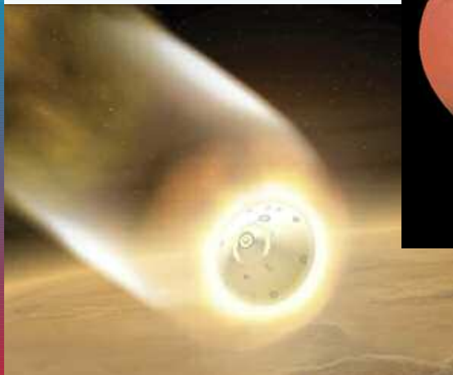
An aeroshell, along with a precise angle of entry, will protect Spirit and Opportunity from burning up as they screech into the Martian atmosphere from interplanetary space. Illustration: JPL/NASA
