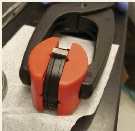
Right and below: This set of three pictures shows the process of attaching titanium cleats, four of which hold the carrier and its lid together. Such a brute-force technique is used deliberately. The cleats actually embed in the Delrin (black plastic) when they are hammered down, increasing their grip.
