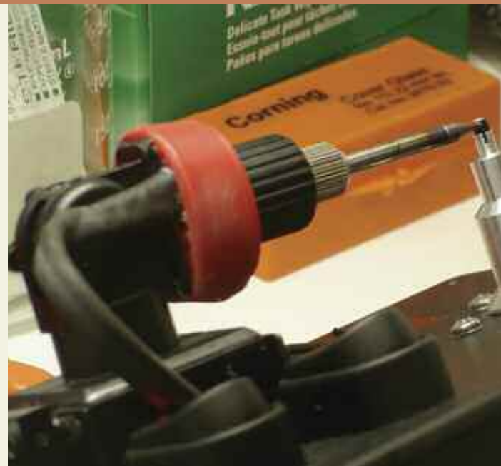
Inside a glove box filled with the inert gas argon, each vial is heat sealed using a specially designed machine. Prior to sealing, each vial is opened and exposed to the argon, then closed for sealing.
