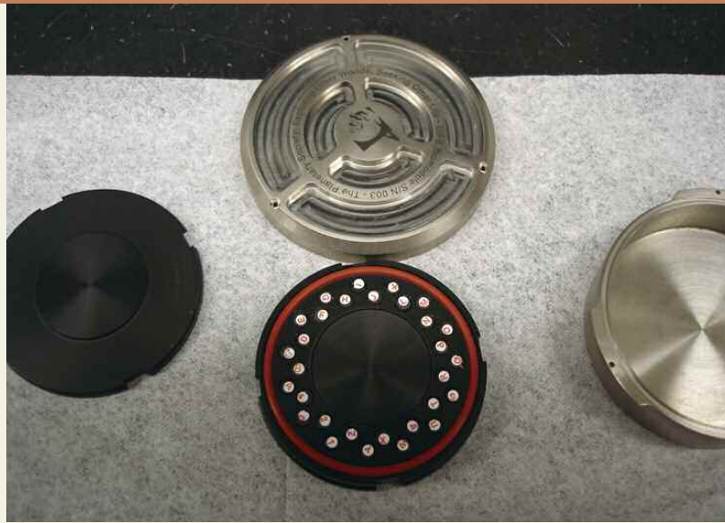
This image shows a filled LIFE biomodule carrier, lid, and titanium outer cases. Individual vials are labeled and color coded differently for each biomodule. The reddish-colored item is a silicone O-ring. It is one of many different seals used in the biomodule for redundancy.
