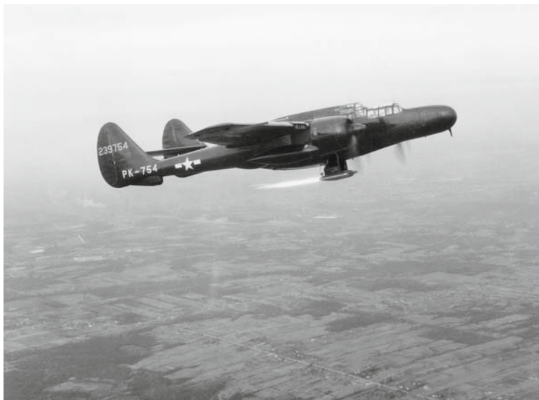
Fig. 8.3 Ramjet technology is not new. This Northrup P-61 Black Widow is flight-testing a subsonic ramjet engine slung beneath (courtesy NASA)
