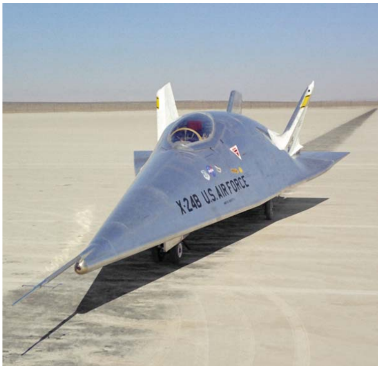
Fig. 1.19 The shape of future spaceplanes? The X-24B “flying flatiron” on lakebed, Edwards AFB, California in 1973 (courtesy NASA)
