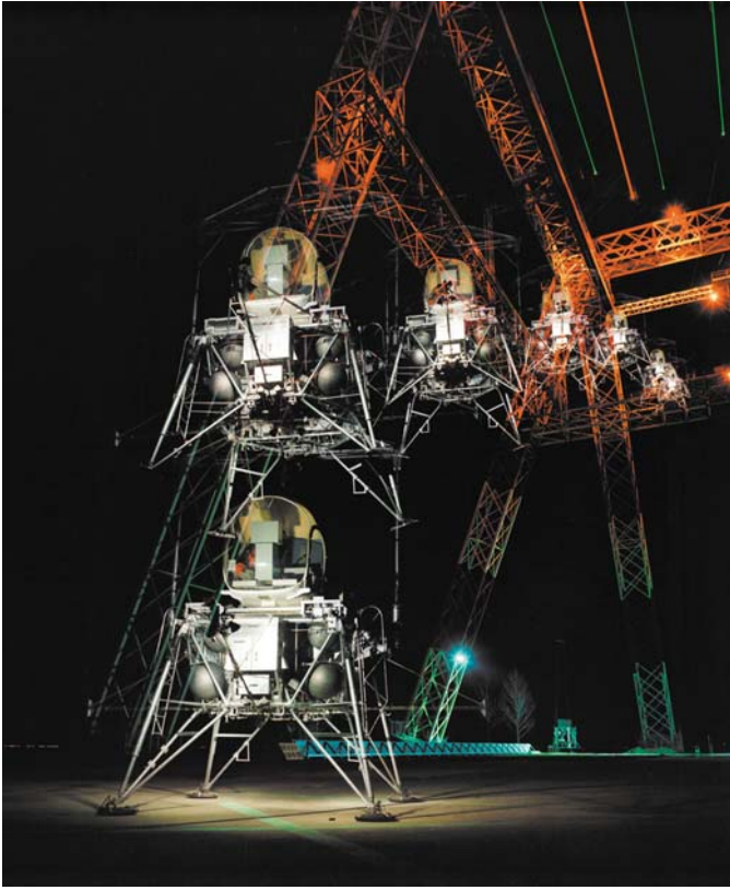
Fig. 10.4 Multiple exposure photograph showing how the Lunar Module approached its touchdown zone, hovering briefly over the landing point before settling to the surface (courtesy NASA)
