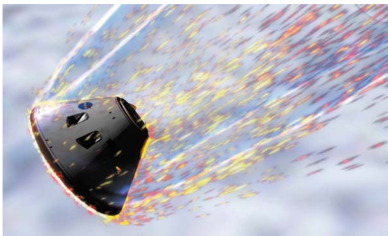
Fig. 10.11 The Orion Crew Capsule enters Earth's atmosphere prior to splashdown at sea or "bump-down" on dry land. Either way, large parachutes are required because the return module has no wings (courtesy NASA)
