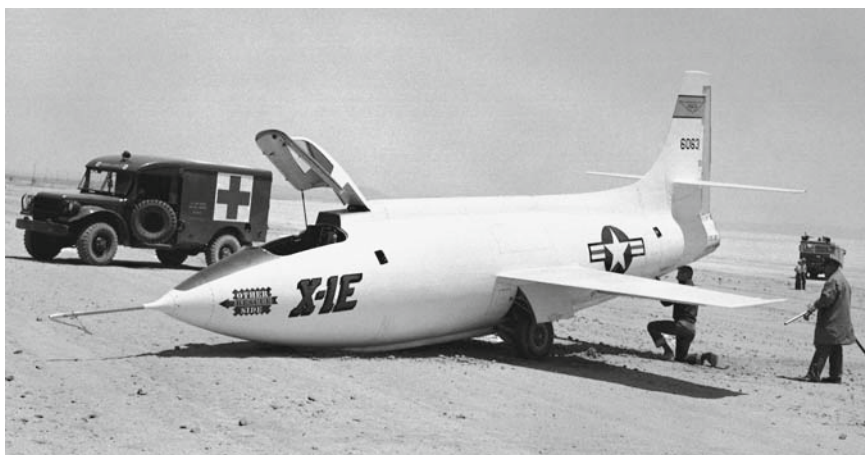
Fig. 9.7 Rocketplanes might trip up, but they do not tip over. Here, the nose gear of the X-1E has collapsed on landing at Rogers Dry Lake in June 1956. The research aircraft was easily repaired to fly again. See also Fig. 2.5 (courtesy NASA)
