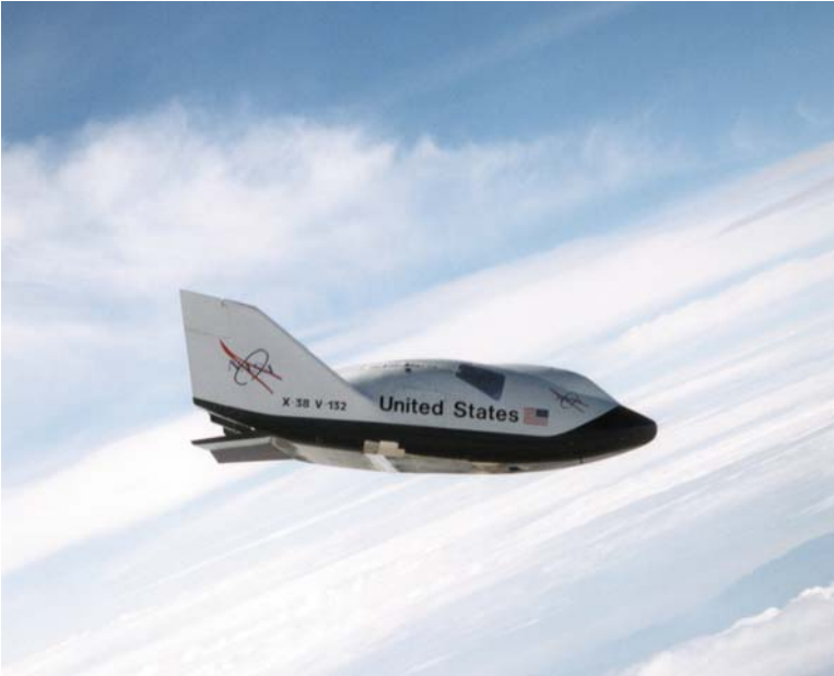
Fig. 2.1 The prespaceplane X-38 lifting body makes a controlled gliding descent after being released from its B-52 “mothership” (courtesy NASA)
