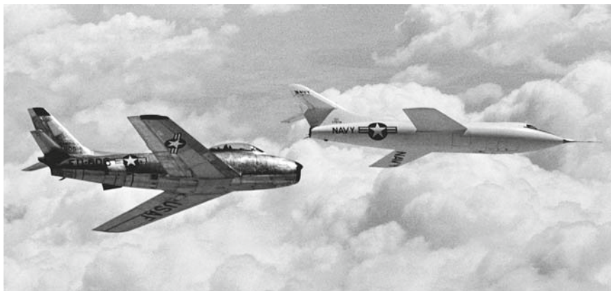
Fig. 9.6 Douglas D-558-2 Skyrocket in flight with F-86 chase plane, during the mid-1950s. The post-war years saw a rapid and continual improvement in airplane and rocketplane designs, exemplified here by the recently introduced swept wings of both aircraft (courtesy NASA)
