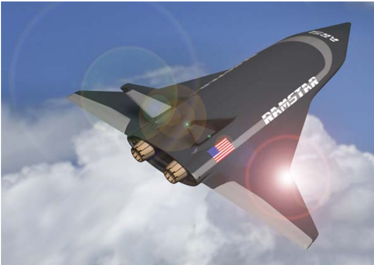
Fig. 12.3 The Ramstar Orbital Spaceplane may utilize a boron slurry in a wide-range ramjet, or use a combined-cycle turbojet/scramjet or hypersonic wave engine (courtesy Aerospace Research Systems, Inc.)
