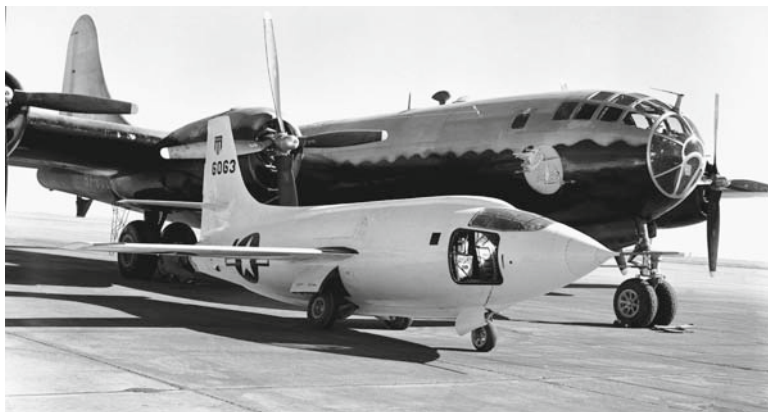
Fig. 1.9 The X-1 “baby” rocketplane with its B-29 mothership, “Fertile Myrtle.” See the stork carrying the baby on Myrtle’s nose (courtesy NASA)
