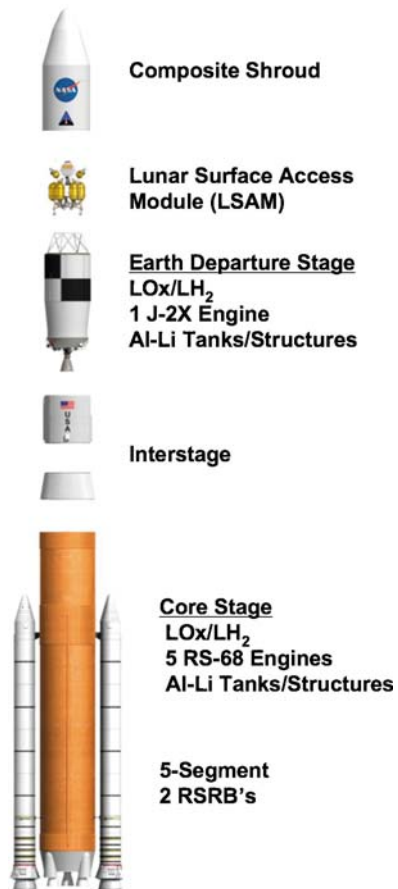
Fig. 10.7 Ares V unmanned rocket, used to launch heavy loads, including Lunar transfer stages and Moon landers. The smaller Ares I (Fig. 2.7) will launch astronaut crews (courtesy NASA)
