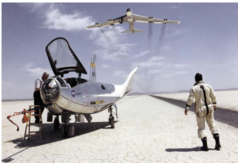
Fig. 1.17 Research pilot Bill Dana and HL-10 on lakebed with B-52 flyby. The HL-10 was the fastest and highest of the lifting bodies, and was judged to be the best handling of the three original heavyweight lifting bodies – the M2-F2/F3, the HL-10, and the X-24A. Compare this photo with Fig. 1.1 (courtesy NASA)
