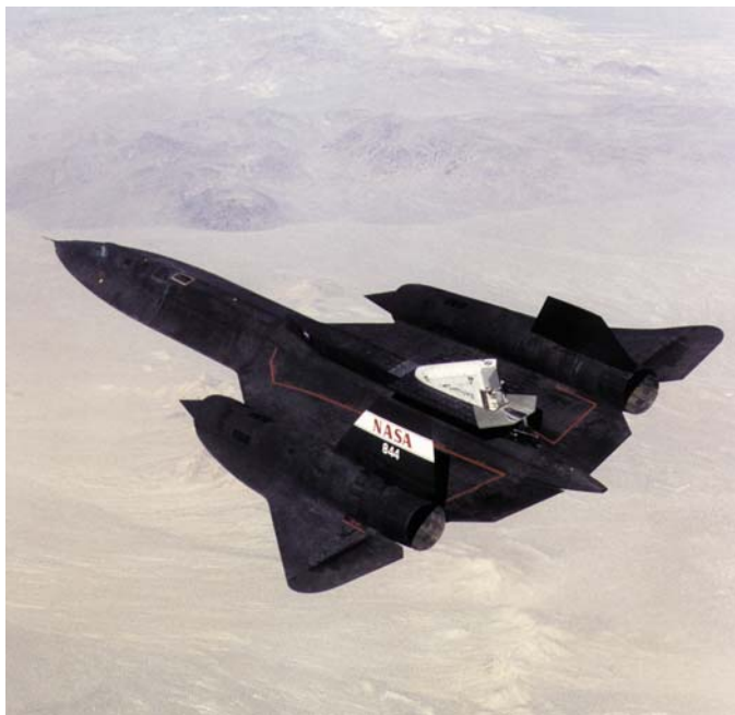
Fig. 8.1 SR-71 Blackbird flight-testing linear aerospike rocket engine (courtesy NASA)
