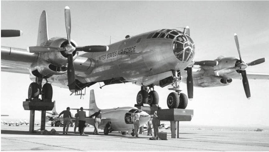
Fig. 11.5 Only baby spaceplanes are carried by their mothers. This is the X-1-3 being carefully mated to an elevated EB-50A Superfortress. A typical government operation (courtesy NASA)
