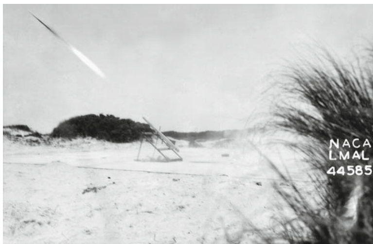
Fig. 4.1 Small 3.25-in. ballistic missile rapidly accelerating skyward from NACA’s Wallops Island facility on June 27, 1945 (courtesy NASA)
