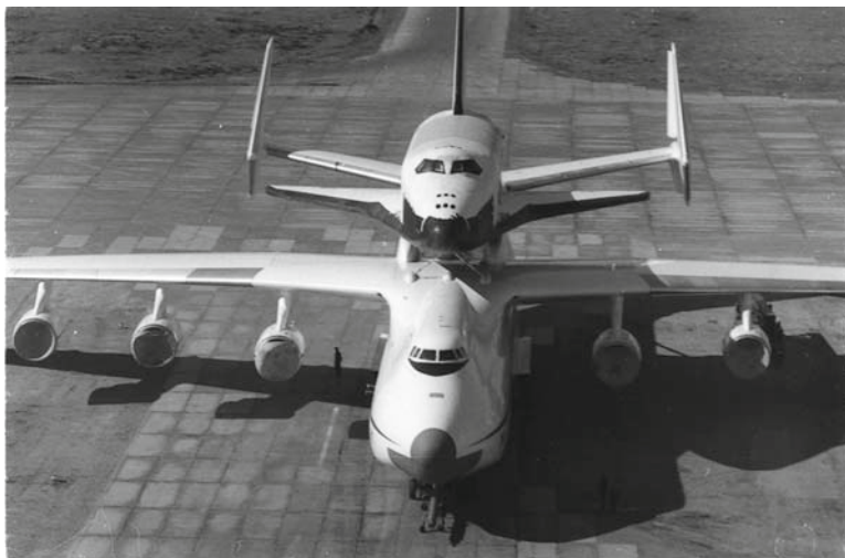
Fig. 7.6 Buran , mounted to its Antonov transport aircraft. Although Buran could be fitted with its own jet engines, the piggyback method was also used (courtesy www.buran-energia.com )
