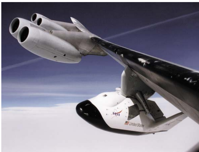
Fig. 3.6 Baby spaceplane X-38 cradles under the wing of its "grandmother" B-52 (courtesy NASA)
