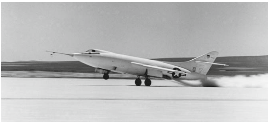
Fig. 5.9 Douglas Skyrocket takes off with small “jet assisted take-off” rockets in 1949 (courtesy NASA)
